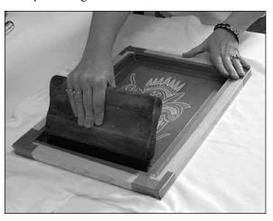
c. Holding the squeegee at a 45 degree angle, pull the line of ink across the image. It may take a little experimenting to find the correct amount of pressure when screening the ink. You may want to have
